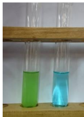
Figure 6: The resulting green solution (left) of copper(II) salicylaldehyde ( C_{14}H_{12}CuO_4 ) complex and the original blue copper(II) sulphate ( CuSO_4 ) solution.
