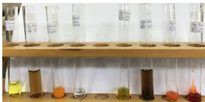
Figure 4: 4 samples of aqueous layer and organic layer of distillate in LHS and RHS. Samples of both layers were tested by, (starting from left) \text{FeCl}_3 with \text{HCl} , \text{FeCl}_3 , 2,4-DNPH and conc. \text{H}_2\text{SO}_4 (right) respectively.
